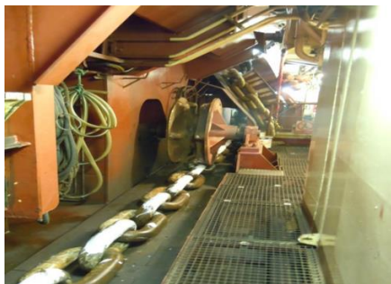
Transporting chains to DSV for offshore installation and marking chain to facilitate offshore installation
