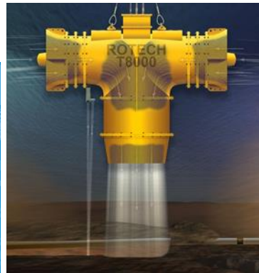
Jetting by Mass-flow Excavator of backfill cover on existing pipeline to facilitate cutting, lifting and above-water tie-in between new and existing pipeline segments
