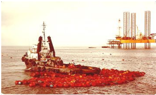
Collection of stripped buoyancy drums for delivery to collection site onshore
