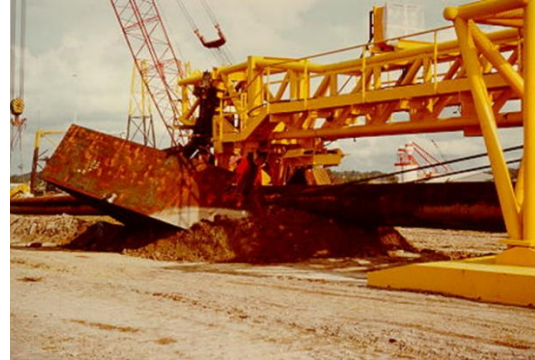
Concept for post-trenching using the plough & onshore testing and adjustment of procedure prior to offshore deployment
