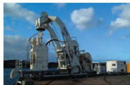
↑ Launching Frame with Heave Compensator
