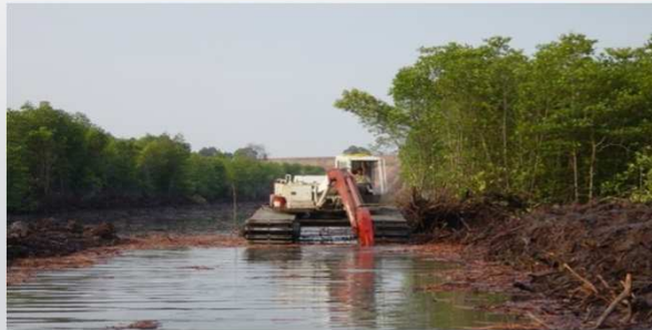
Buoyancy Drums to Provide Positive Buoyancy
