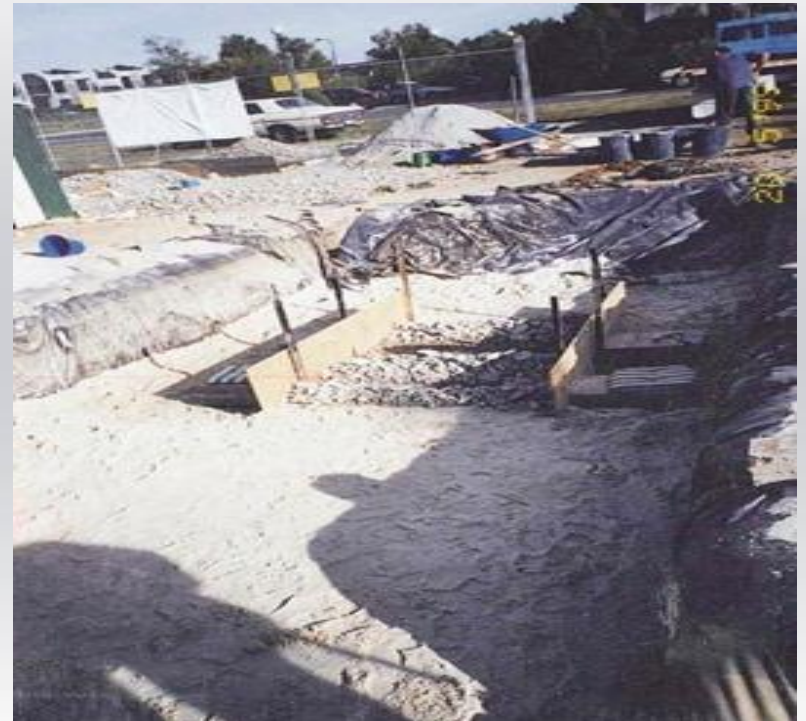
Preparation of prototype model for anchor drag test
