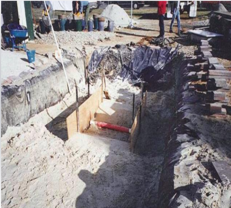
Preparation of prototype model for anchor drag test
