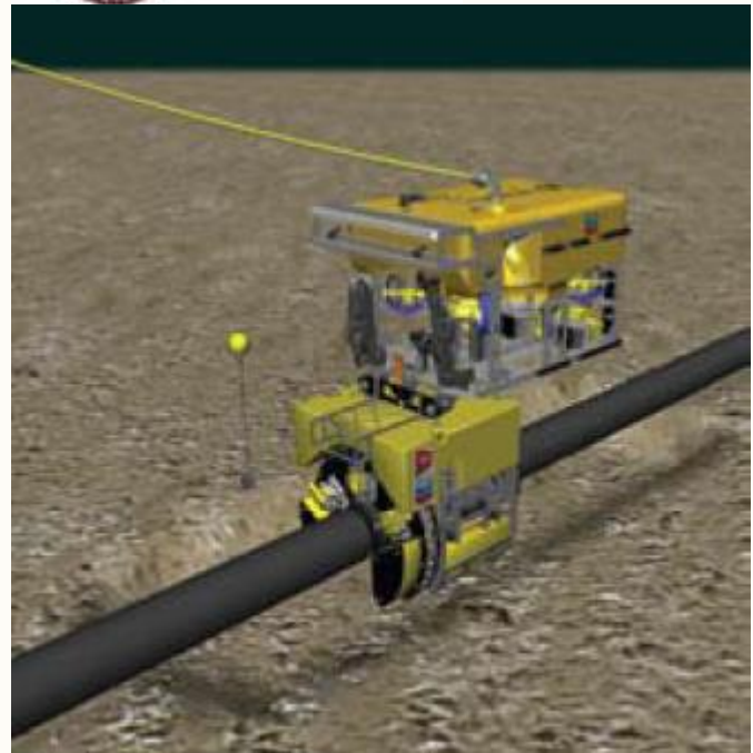
Pipeline Preparation Tool on Damaged Pipe and Operated by ROV
