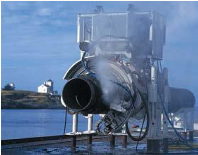
Typical Concrete Coating Removal Tools: (L) STATOIL and (R) CAPE
