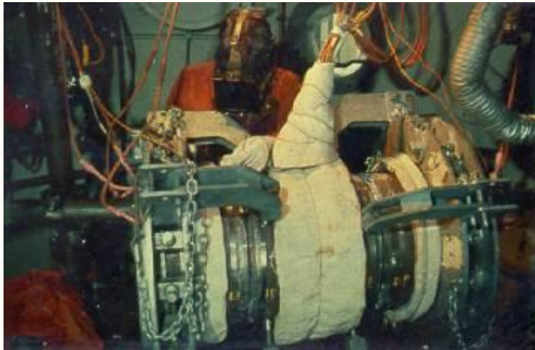
Welding trials ongoing in the work chamber of a Hyperbaric centre (L) and Saturation Control (R)
