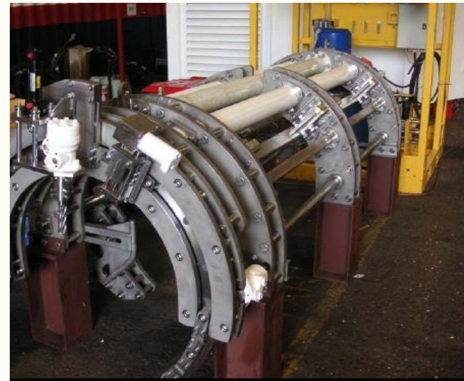
Typical Concrete Coating Removal Tools: (L) STATOIL and (R) CAPE
