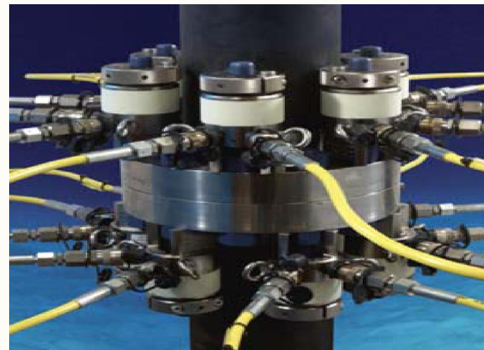
Underwater bolt tightening using Hydratight bolt tensioning equipment.
