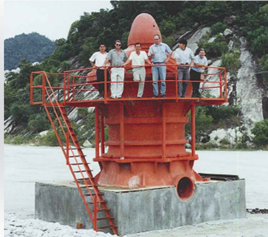
Above: Dis-used Rock Crusher - Note its size
