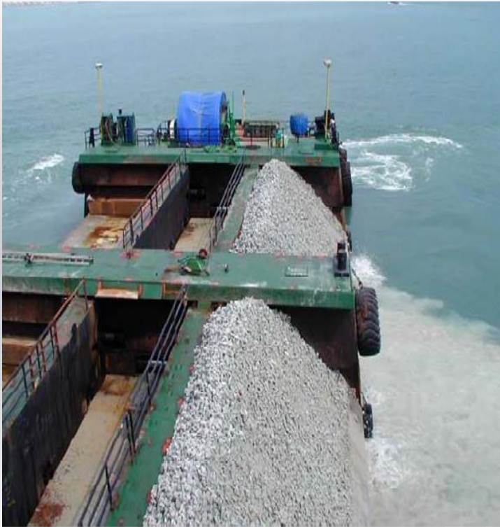
(L) Side Stone Dumping Vessel; (R) Fall Pipe Stone Dumping Vessel
