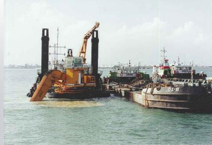
Van Oord's Backhoe Dredger "Ave Caesar" dredging rocky seabed in Singapore & 2 no. hopper barges for disposal of spoils
