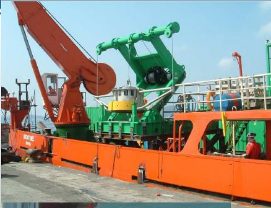
SeaVator Mass Flow Excavator with V-jet system (left)
