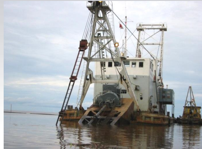
Shallow water cutter suction dredger
