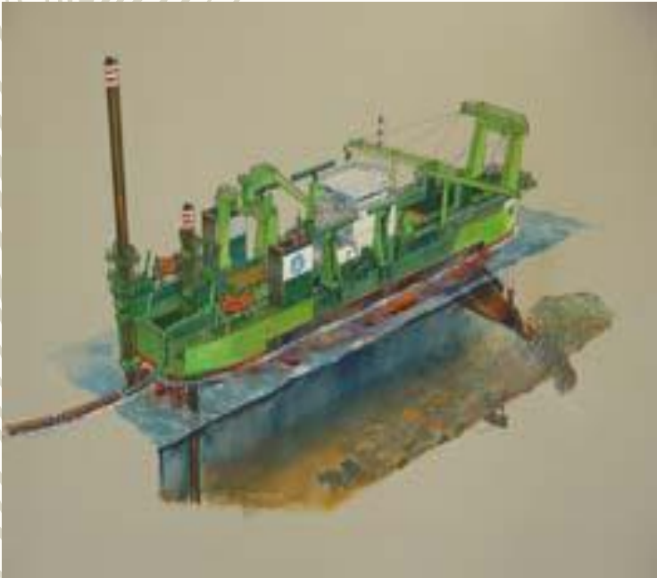
Tideway Cutter Suction Dredger "d'Artagnan" (dredging up to 30m depth)
