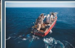
Reel-lay Method of Installation
