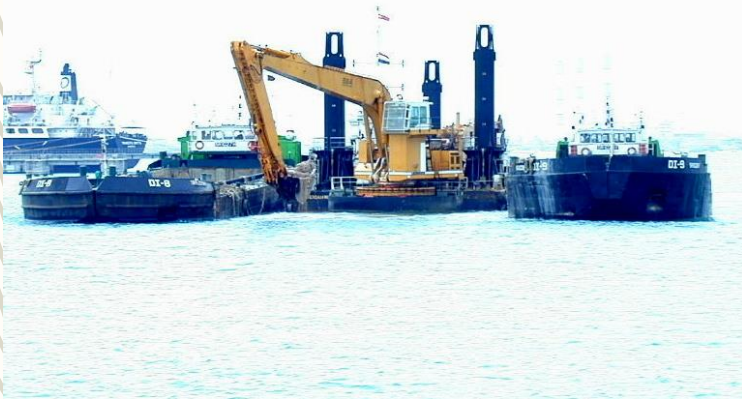
Van Oord's Backhoe Dredger "Ave Caesar" dredging rocky seabed in Singapore & 2 no. hopper barges for disposal of spoils
