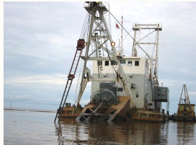
Shallow water cutter suction dredger
