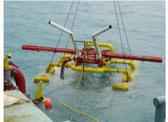
Closer View of Jetting Claw, Showing Nozzles and Eductors
