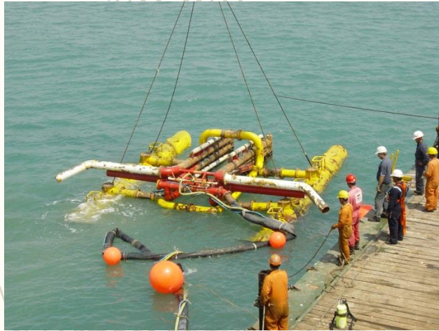
Closer View of Jetting Claw, Showing Nozzles and Eductors
