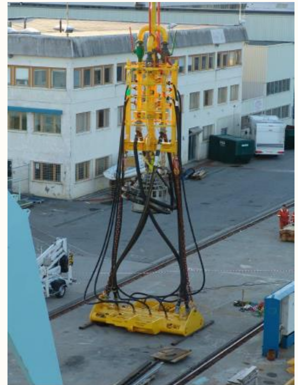
ClayCutterX can cut 5m wide trench in soils up to 500kPa
