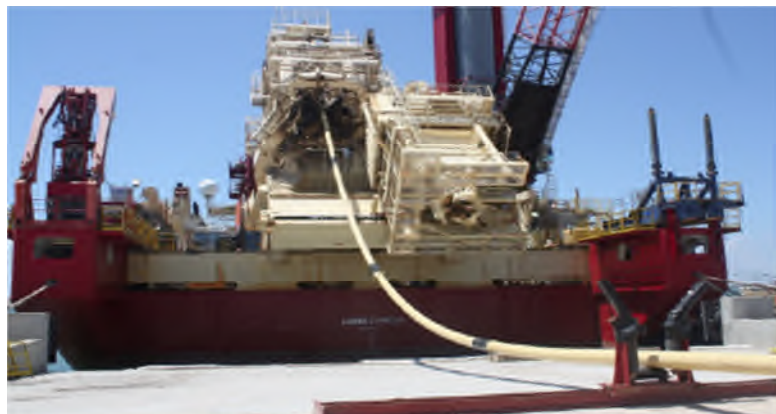
Figure 15 Reel Lay Typical Process (Clockwise from Top Left): (a) Welding and NDT within Spool base; (b & c) Reeling onto Reel Vessel; (d) Packing onto carousel.
