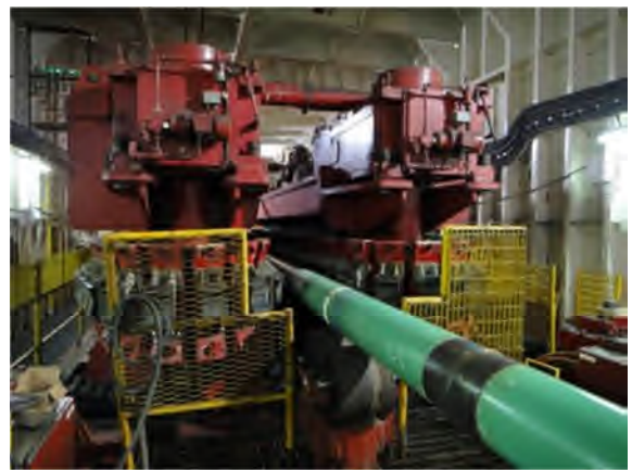
Figure 4 S-Lay Typical Process (Clockwise from Top Left): (a) Welding; (b) Welding Inspection/ Test; (c) Going through Tensioner; (d) Pipeline Going through Stinger before Lift-Off
