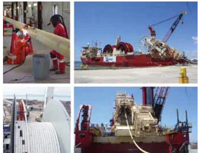
Figure 13: Reel Lay Typical Process (Clockwise from Top Left): (a) Welding and NDT within Spool base; (b & c) Reeling onto Reel Vessel; (d) Packing onto carousel.
